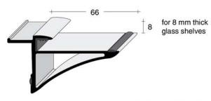
HV8 load behaviour is optimal if the support is used for the whole length of the glass
